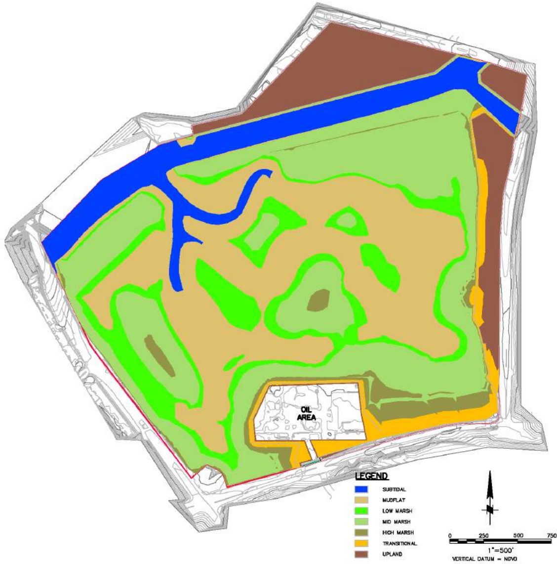
Figure 7-93. Habitat Elevation Bands, Moderate Alteration, Northern Area – Sea Level +1.5 ft
