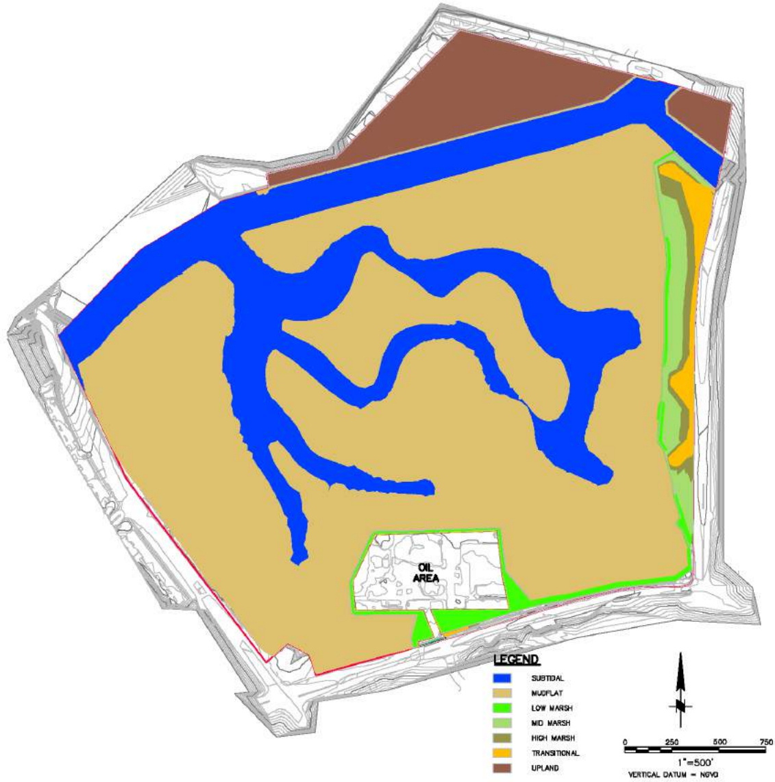
Figure 7-97. Habitat Elevation Bands, Moderate Alteration, Northern Area – Sea Level +5.5 ft
