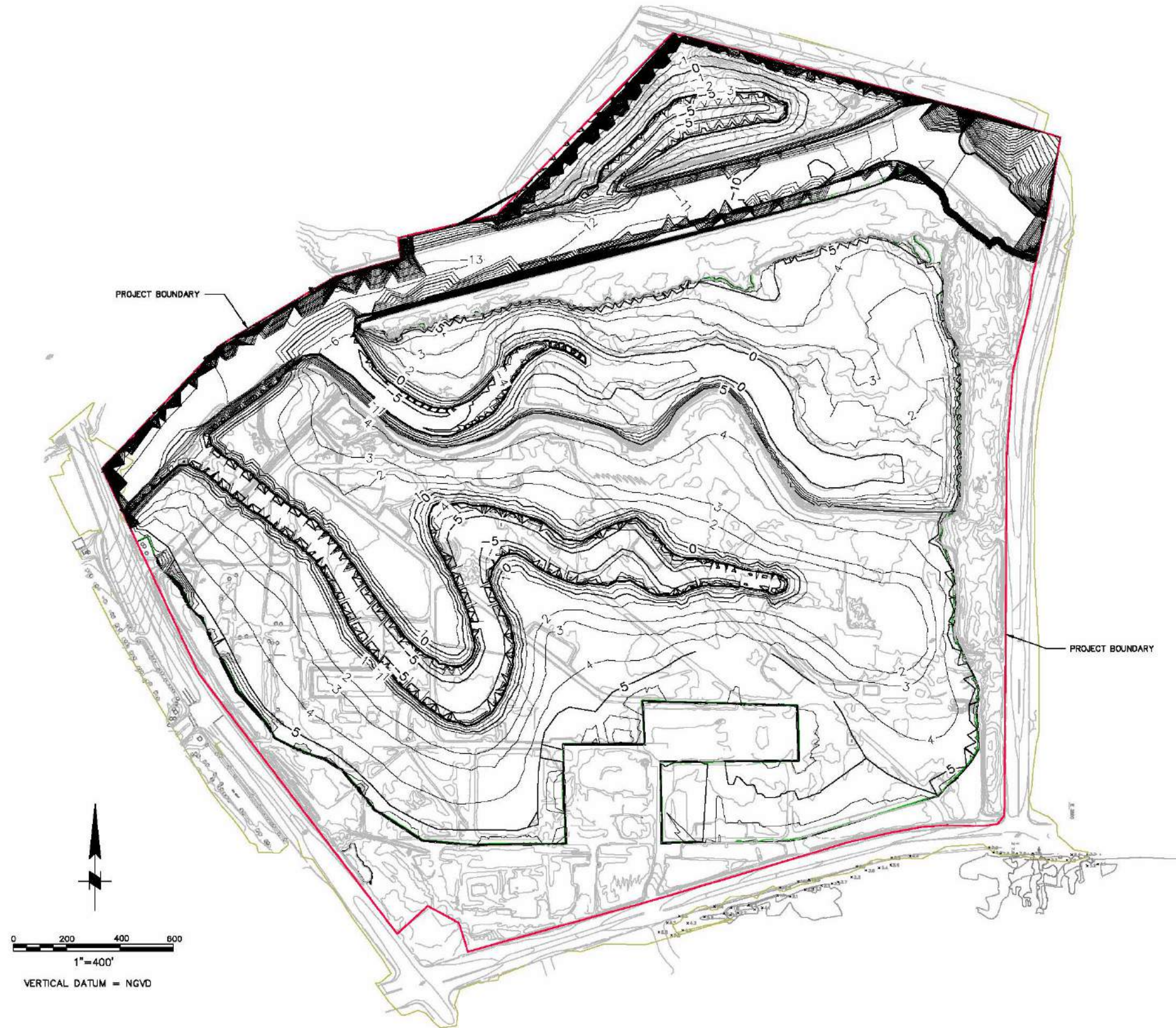
Figure 7-101. Conceptual Grading, Maximum Alteration, Northern Area
