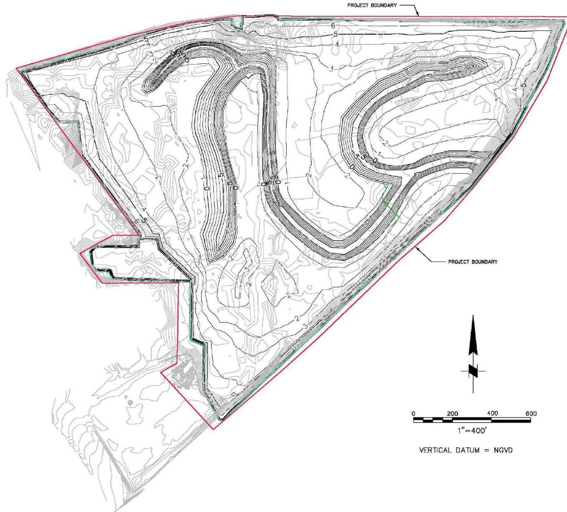
Figure 7-65. Conceptual Grading, Moderate Alteration, Central Area
