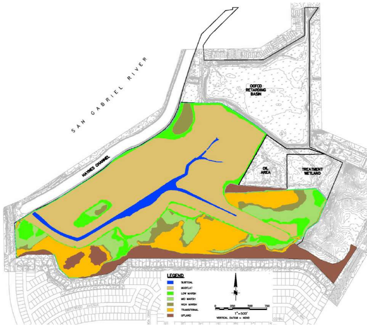
Figure 7-100. Habitat Elevation Bands, Moderate Alteration, Southeast Area – Sea Level +5.5 ft
