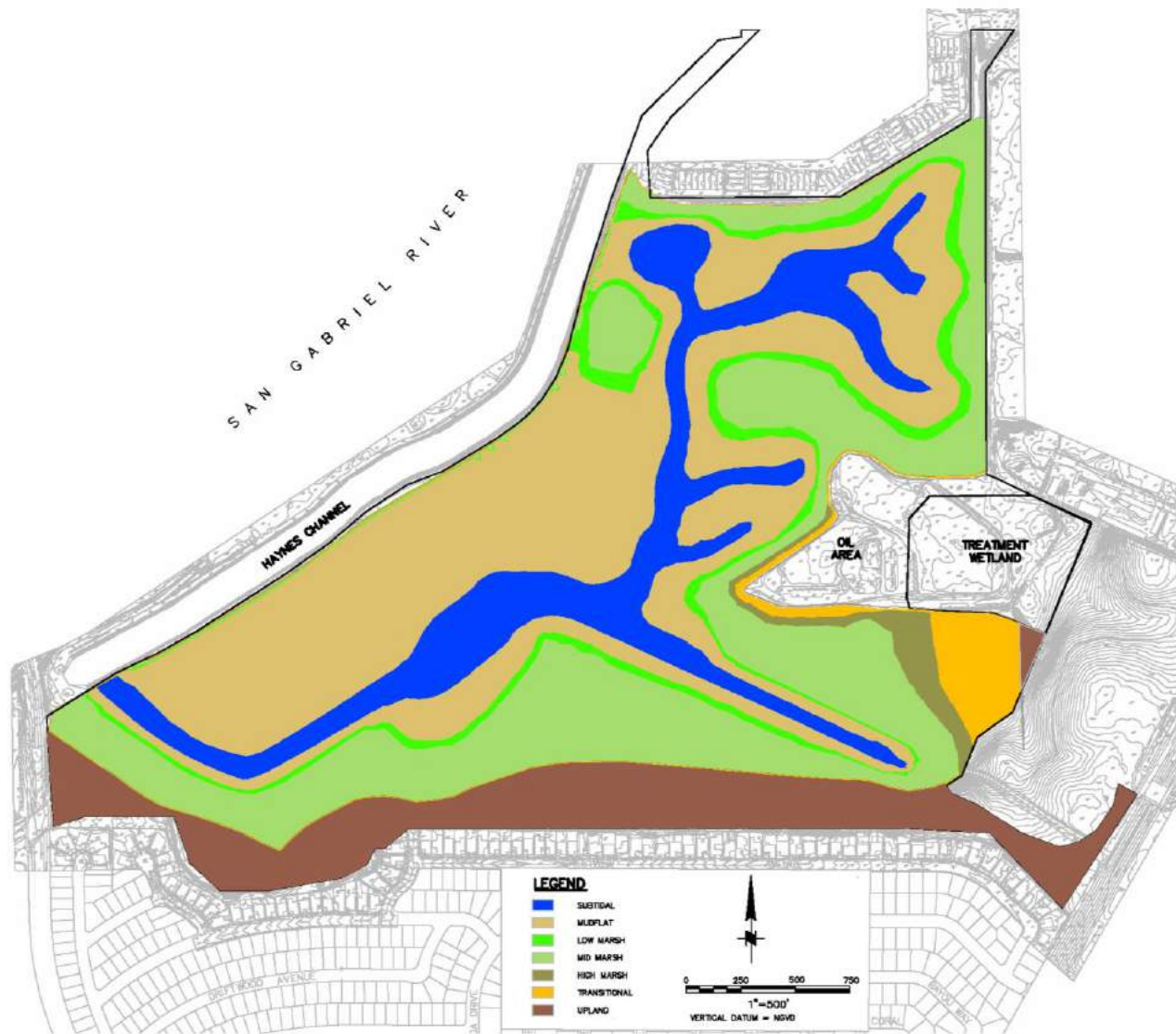
Figure 7-137. Habitat Elevation Bands, Maximum Alteration, Southeast Area, 1.5 Feet of SLR
